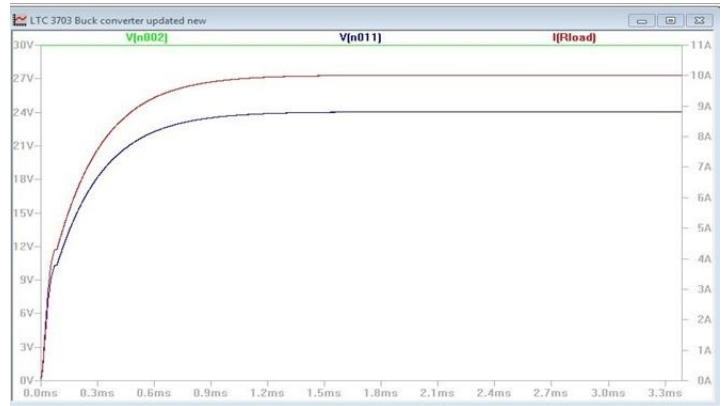
Fig. 5: Output current and output voltage waveform for 30 V
